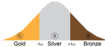
Figure 3. Assignment of Gold (G), Silver (S), and Bronze (B) rankings to a company's KPI assuming that KPI values follow a normal distribution (lower score is better)
